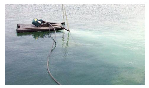
Oxygen injection systems output high-purity oxygen directly into pond water. With source oxygen fed through a hose, this floating unit distributes an oxygen plume in a pond.
