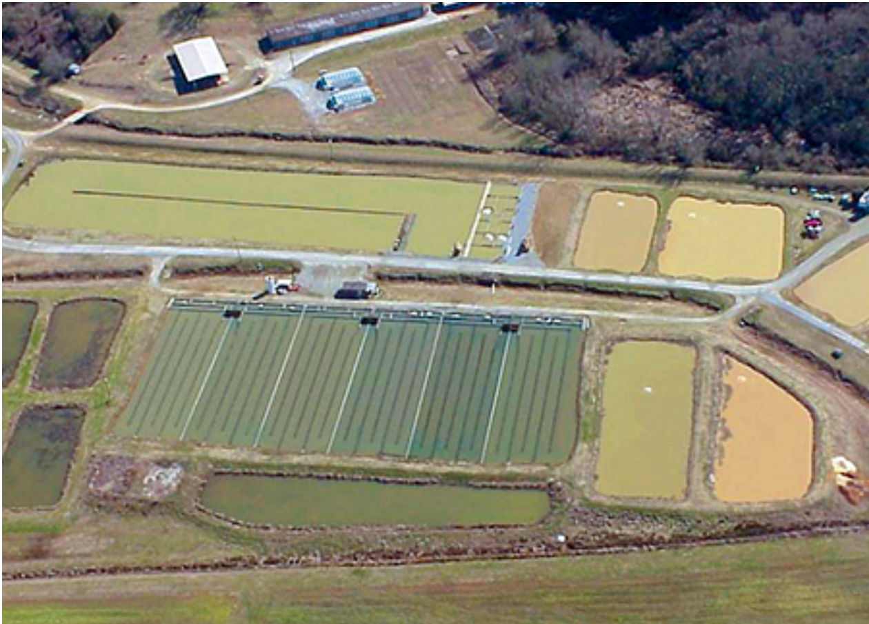
Partitioned aquaculture yields more fish than earthen pond culture while using much less water.
