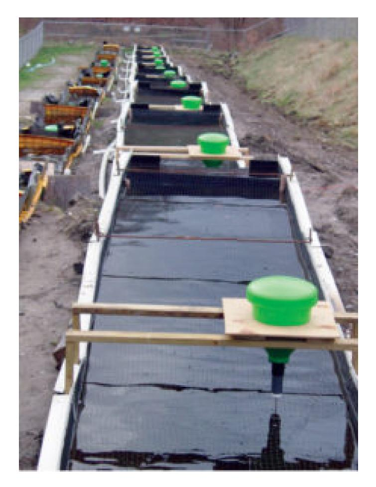
U-shaped plastic tanks cost less to purchase, install and clean than flat-bottom concrete tanks of similar volume.
