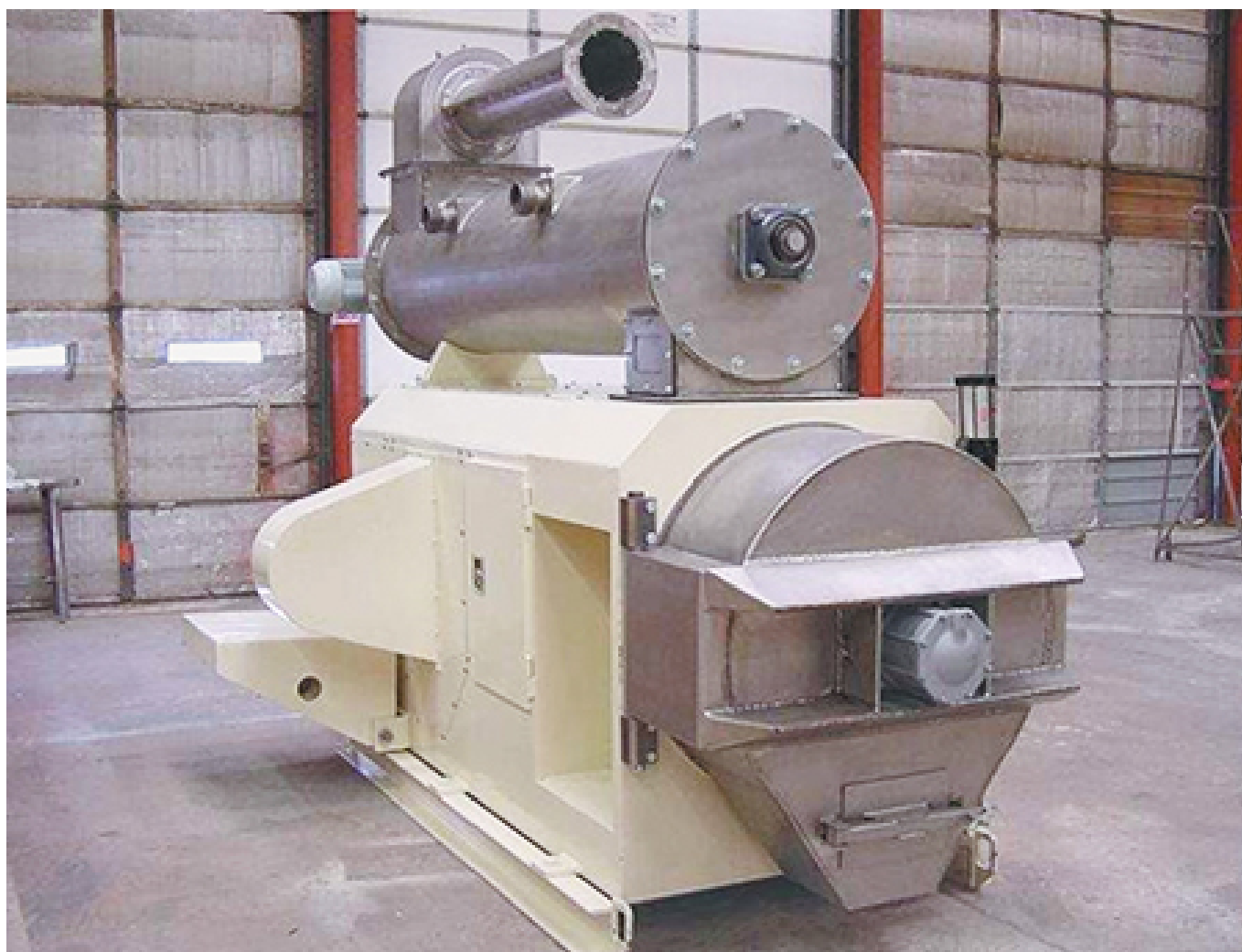
Fig. 1: Integrated pressurized preconditioner and pellet mill. Photo courtesy of Pelleting Concepts International.
