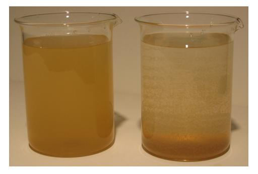
An application of alum cleared the turbid water sample on the right.
