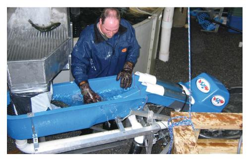
The air-lift fish pump at the left delivers rainbow trout from the culture tank in the rear to the water-filled orientation chamber at front. Fish swim automatically or are slid into the channels that feed into the blue stunning chamber and collection basin at right.
