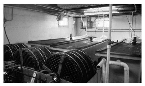
RAS system used for polyculture of Nile tilapia and channel catfish. Note rotating biodisc in foreground.
