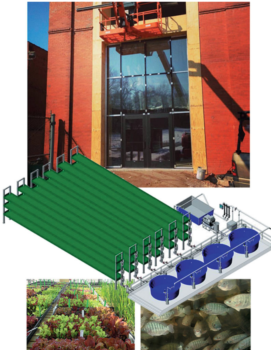
A project under way within a former brewery building in St. Paul, Minnesota, USA, is raising lettuce and leafy greens along with tilapia in an RAS system.
