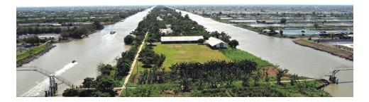
The original DCD farm design incorporated a common canal system that both handled effluents and provided boat access to individual ponds.
