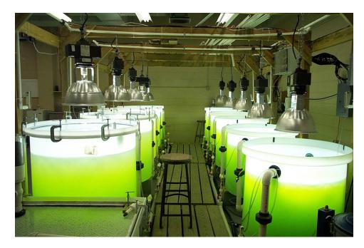
Microalgae was produced in a hydraulically integrated serial turbidostat algal reactor (HISTAR) system, harvested as a paste, refrigerated, and analyzed.
