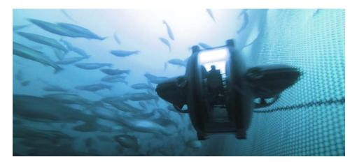
Deep Trekker manufactures portable underwater inspection tools like the DTX2 ROV – an underwater remotely operated vehicle (ROVs)
