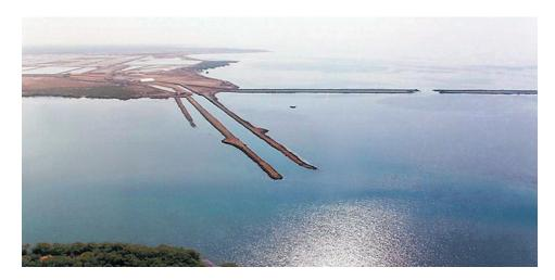
Water is drawn from the Red Sea, then pumped to reservoirs and gravity-fed through concrete canals to the grow-out ponds.
