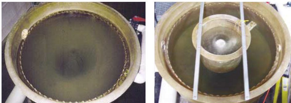
(Left) Fig. 1: As water rotates within a swirl separator, solids removal is mainly gravity-driven. (Right) Fig. 2: Radial-flow settlers are often used to settle microbiological solids during secondary water treatment.
