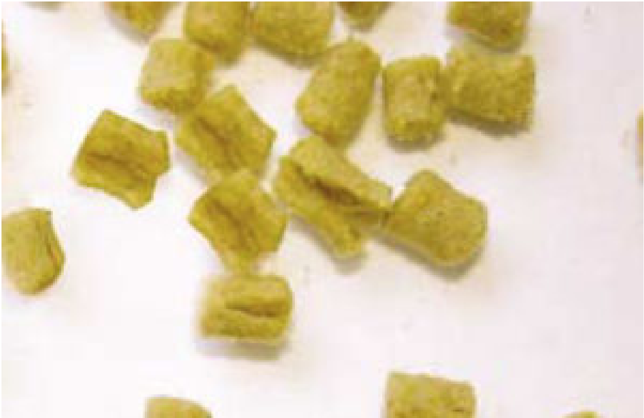
Fig. 2: Pellets produced under medium shear had longitudinal cracks after four hours of immersion.
