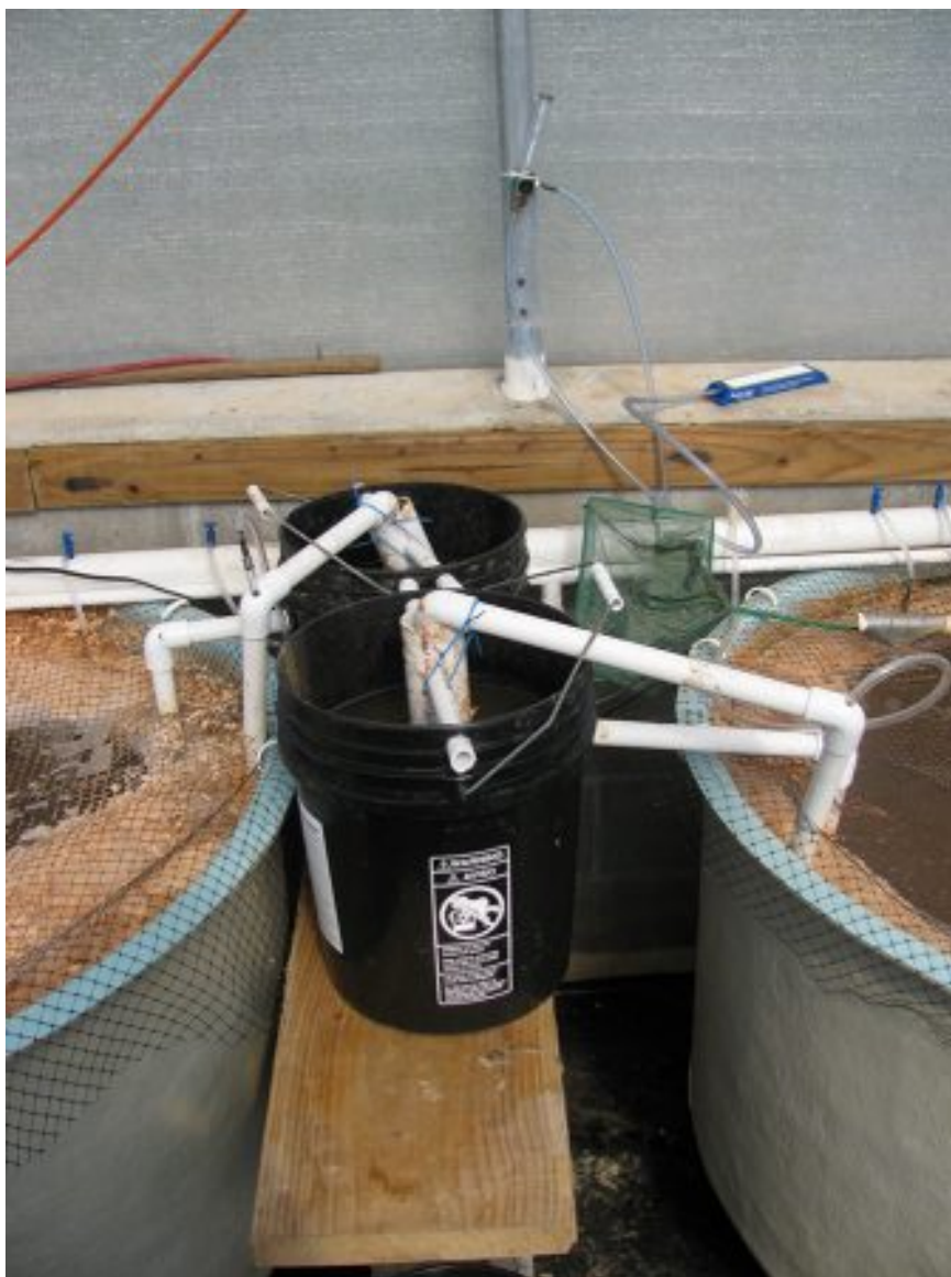
One of the settling chambers used in the study to remove solids.
