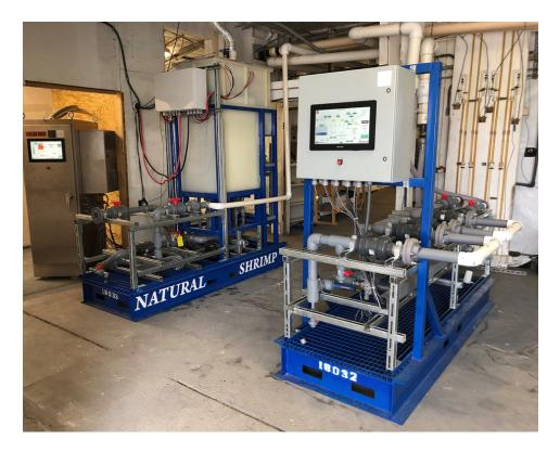
Texas-based company NaturalShrimp uses a light electrical charge, a process called electrocoagulation, to remove and control bacteria, ammonia and other contaminants that hinder shrimp production. Courtesy photo.
