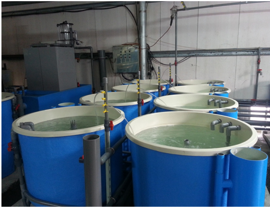
Experimental tanks and the recirculating system used in the study; each tank was set-up with a feces collection column.
