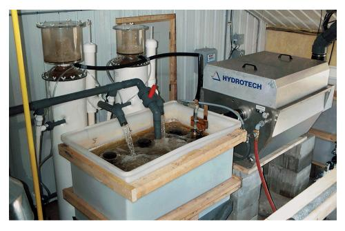
Water that drains from the culture tanks is passed through a drum filter (right), foam fractionators (columns in rear) and heating tank (foreground) before reuse.
