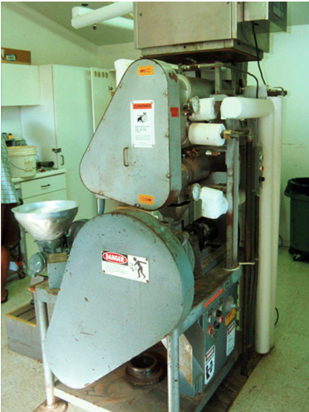
A laboratory pellet mill was used to prepare the control diets.
