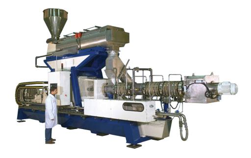
Advances in twin-screw extruder technology are quickly leading to greater control and flexibility in aquafeed manufacturing. Photo courtesy of Clextral Inc.
