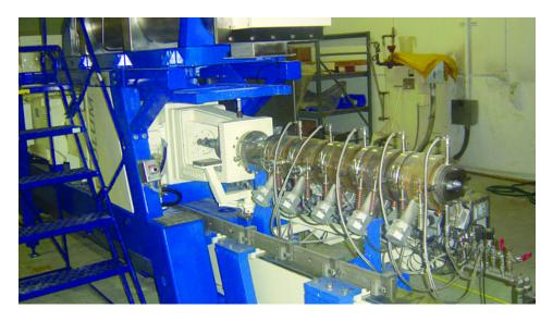
Simpler and less expensive than twin-screw designs, single-screw extruders offer a lesser range of functionality.
