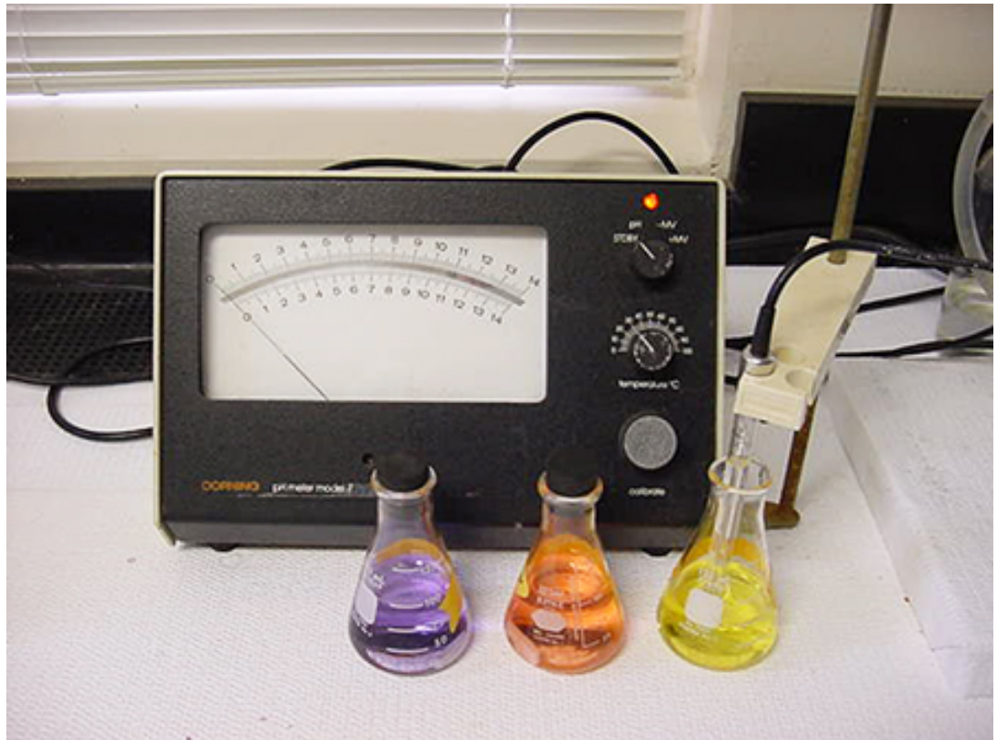
Fig. 3: pH meters with glass electrodes provide the most accurate measurements.
