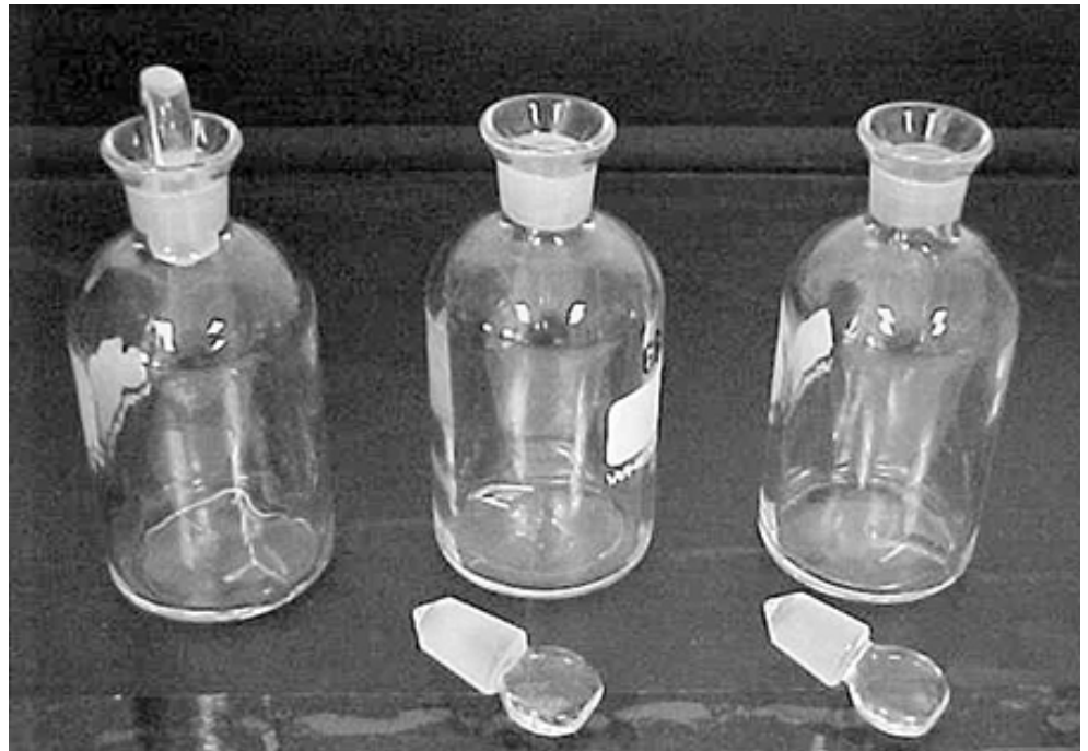
BOD testing begins by placing water samples in sealed bottles under controlled temperature and light conditions.
