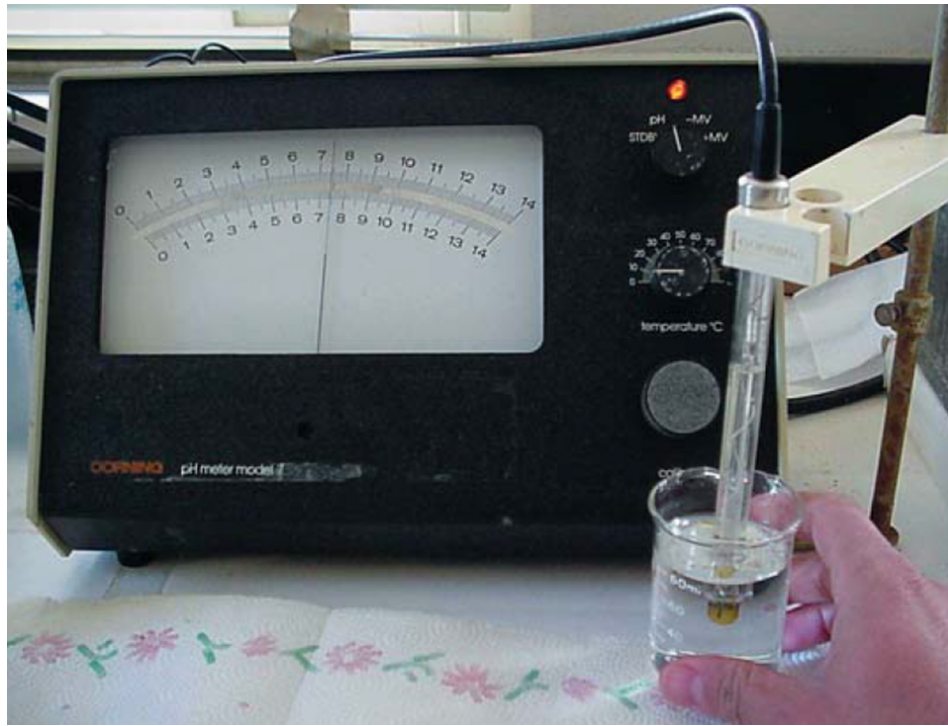
Fig. 2: The only reliable way of measuring pH is with an electronic pH meter.
