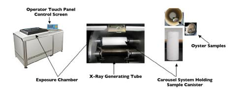
Basic components of an x-ray-generating system.
